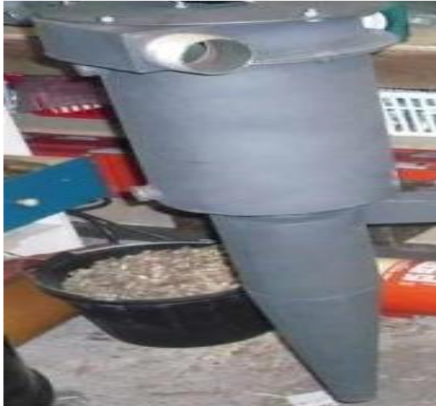
Figure 9 Cyclone is a popular, economical, and effective means of controlling particles. Cyclone can not control alone the stringent air pollution, but functions as precleaners for control devices. [13]
