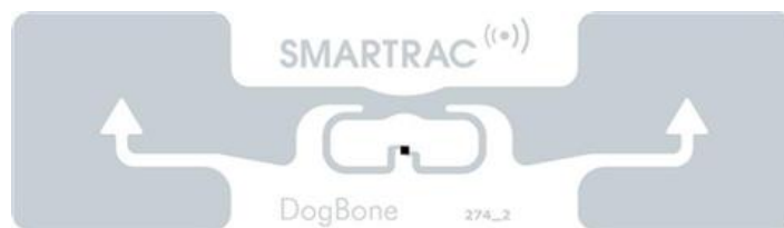
Figure 4. Exemplary SMARTRAC Dogbone RFID paper tag (atlasRFIDstore.com (Ed.) 2017)
