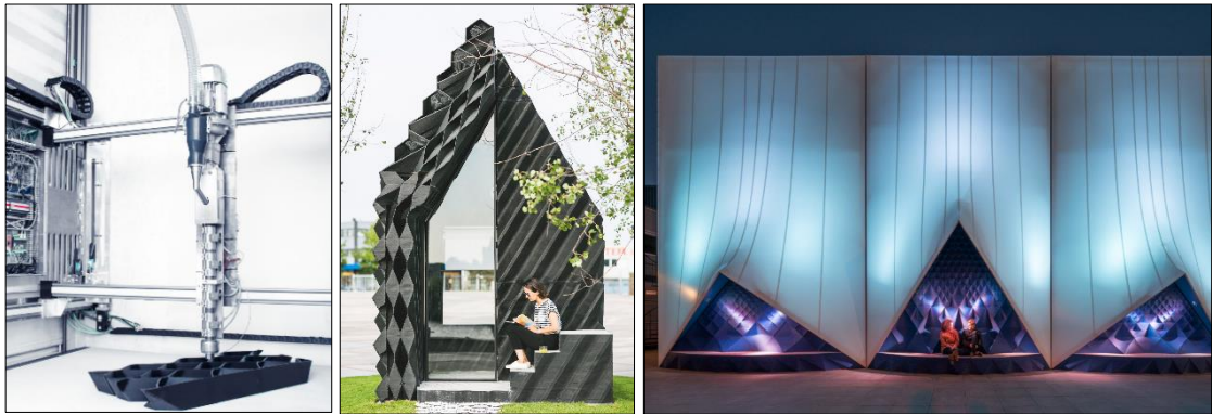
Picture 7. (a) 3D printing canal house nozzle called kamermaker is printing one of cabin piece which will be assembled like a puzzle. Image by demeeuw web magazine. (b) Printed 8 m 2 urban cabin by DUS architects team through kamermaker in Amsterdam. Image by: Sophia van den Hoek (c) DUS Architects has mixed 3D-printed bioplastic with a tensile fabric structure to build a sculptural facade for the building where European Union meetings will take place soon. Image by DeZeen.com, Dutch EU building features a facade combining tensile fabric and 3D-printed bioplastic, 2016.
