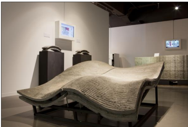
Picture 3. 3D Concrete printing developing large scale additive processes for the manufacture of building components. Developed at the additive manufacturing research group at Loughborough University. Image source: Loughborough University, 3D Concrete Printing: an innovative construction process buildfreeform.com/index.php
