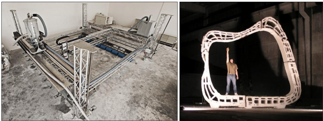
Picture 4. (a) The second-generation of D-Shape machine was the world's first large scale 3D printing technology. Developed by civil engineer Enrico Dini. Image by D Shape. (b) Villa Roccia and Gaudi Tribute one of the D-Shape™ project. The building blocks were 3D Printed and temporary assembled. The local authority did not give the permission to build and the project was terminated. Image by Monolite UK Ltd.
