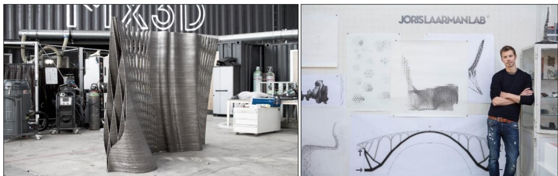
Picture 9. (a) Final design of metal bridge is started to print by MX3D in Amsterdam, the print will be ready early 2018. Image by MX3D. (b) In his lab in Amsterdam, Joris Laarman worked on the first drafts of the metal bridge. Image by: heijmans.nl
