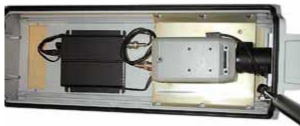
Figure 22. A one – channel video encoder connected to an analog camera (Axis Communications b, 4)
