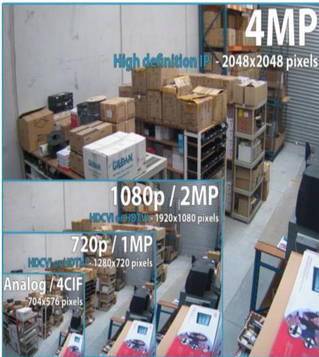
Figure 39. Difference in image quality between analog and IP cameras (website of TRINITY cctv solutions 2017)
