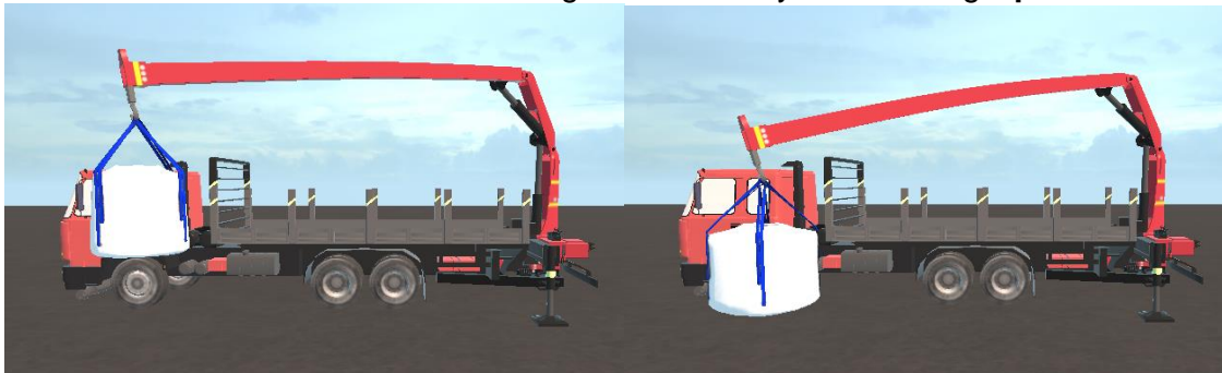
Figure 5: Flexible boom with default bag mass and 1500kg
