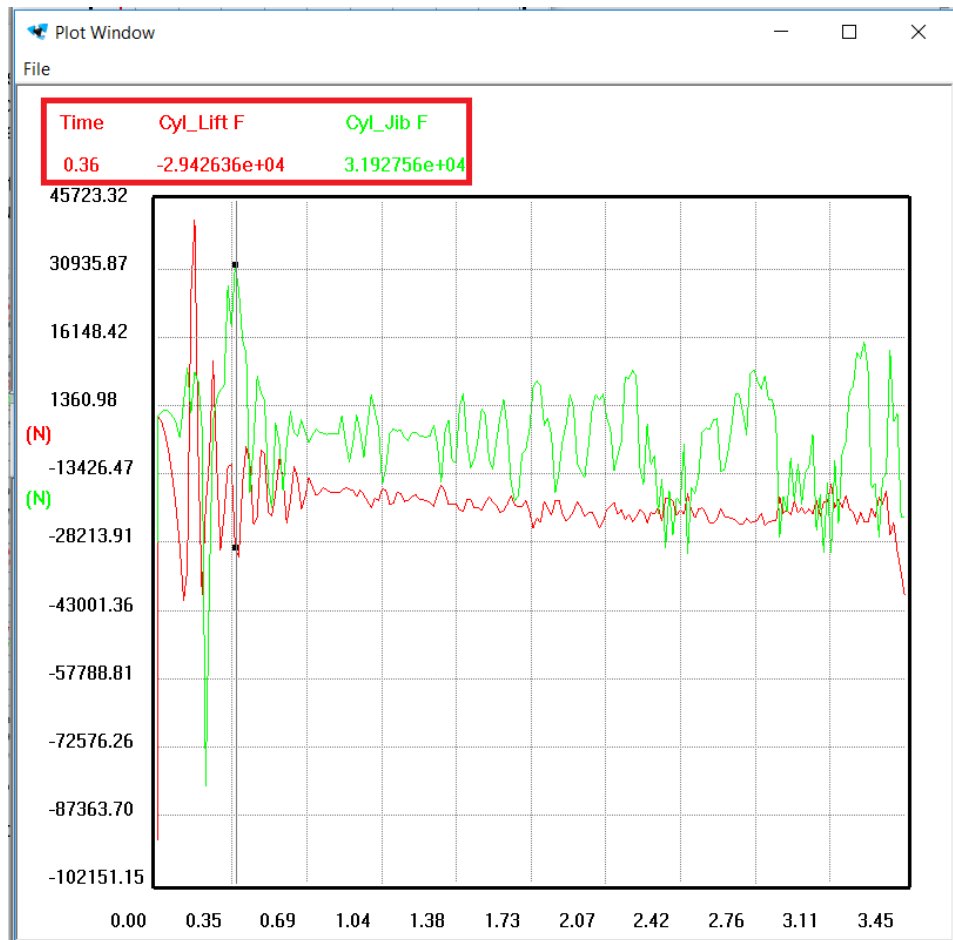
Figure 8: Cylinder lift and cylinder jib forces at 0.36s after the start of the simulation
