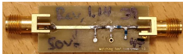
Figure 6. Detector diode circuit with two inductors for input matching.
