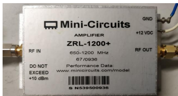
Figure 5. Low Noise Amplifier with 30 dB gain.
