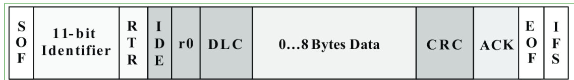
Figure 2. Complete CAN Message Field
