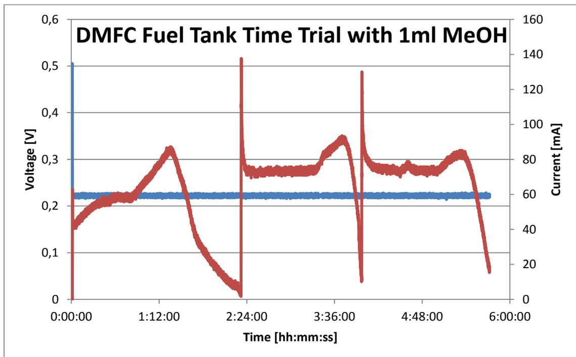
Figure 2: Time based measurement of a DMFC with a 1ml 2M methanol tank connected to it and refilled twice. Voltage is shown in blue and current in red.
