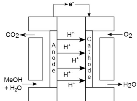
Figure 1: Schematic drawing of the mass transport in a DMFC system.
