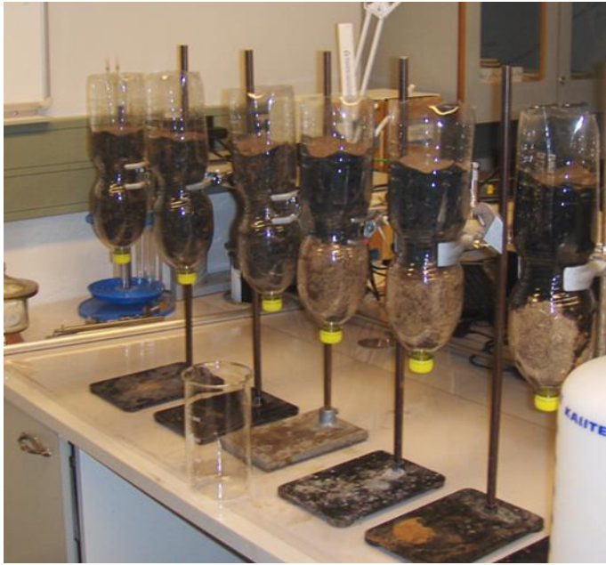
Figure 2. The filter columns being constructed
