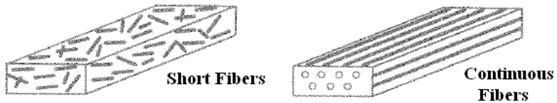
Figure 1.1 Two different kinds of fiber placement in composite material
