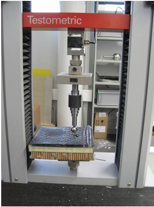
Figure 14.5. The method of compression with testometric machine Authors own work
