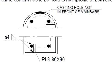
Reinforcement has to be fixed to mainprofile at both ends
