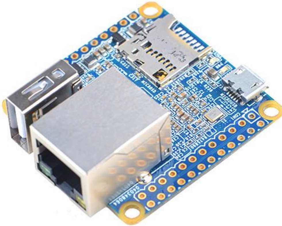
Figure 5. Matchbox-sized SBC with Ethernet and USB connections (Brown 2016)
