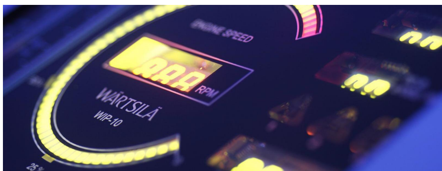
Figure 17. UNIC engine control system. /15/
