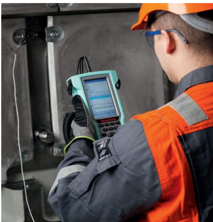
Figure 47. Vibration measurement from a Wärtsilä 32 engine ongoing. /48/
