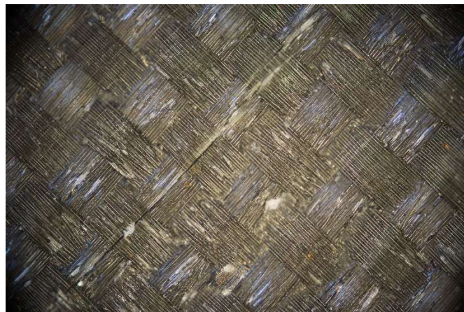
Figure 34. Plain weave microscopic image (top view)
