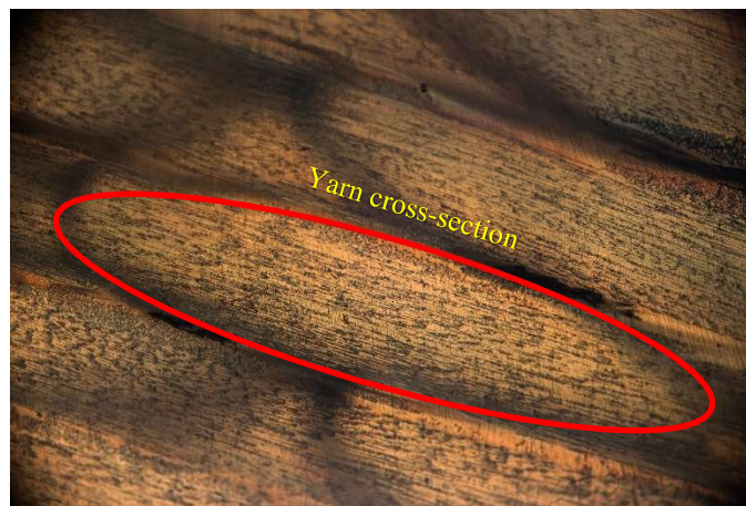
Figure 39. Microscopic image of yarn cross-section (2)
