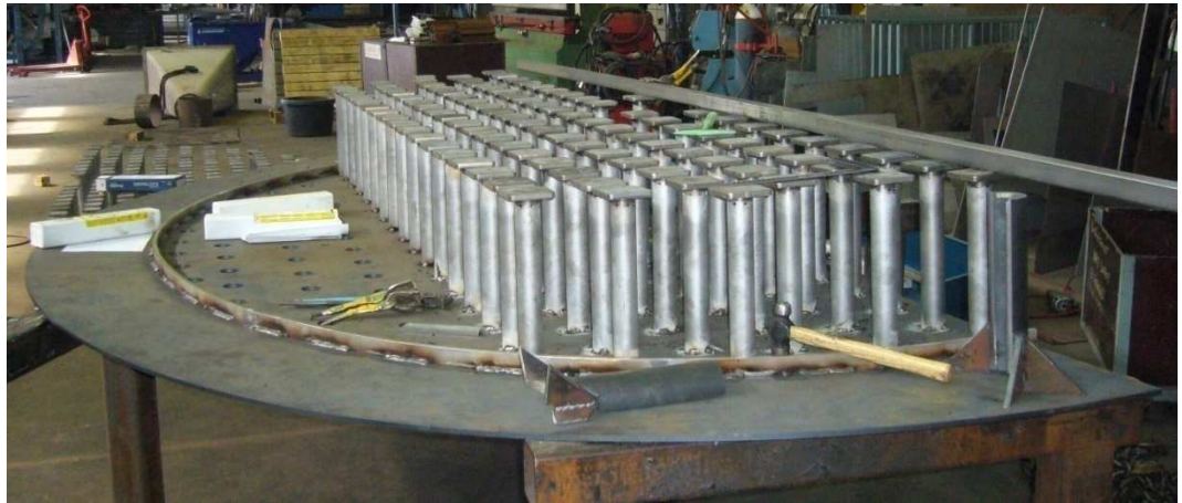
FIGURE 9: Welding assembly of grate parts at Kemas Oy workshop. A jig used is seen in the foreground
