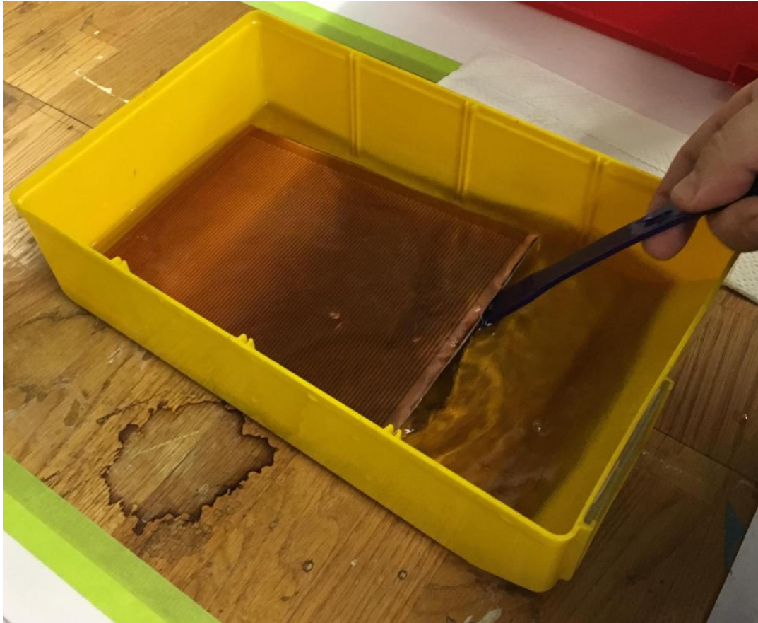
Figure 19. Substrate in the Developer Solution
