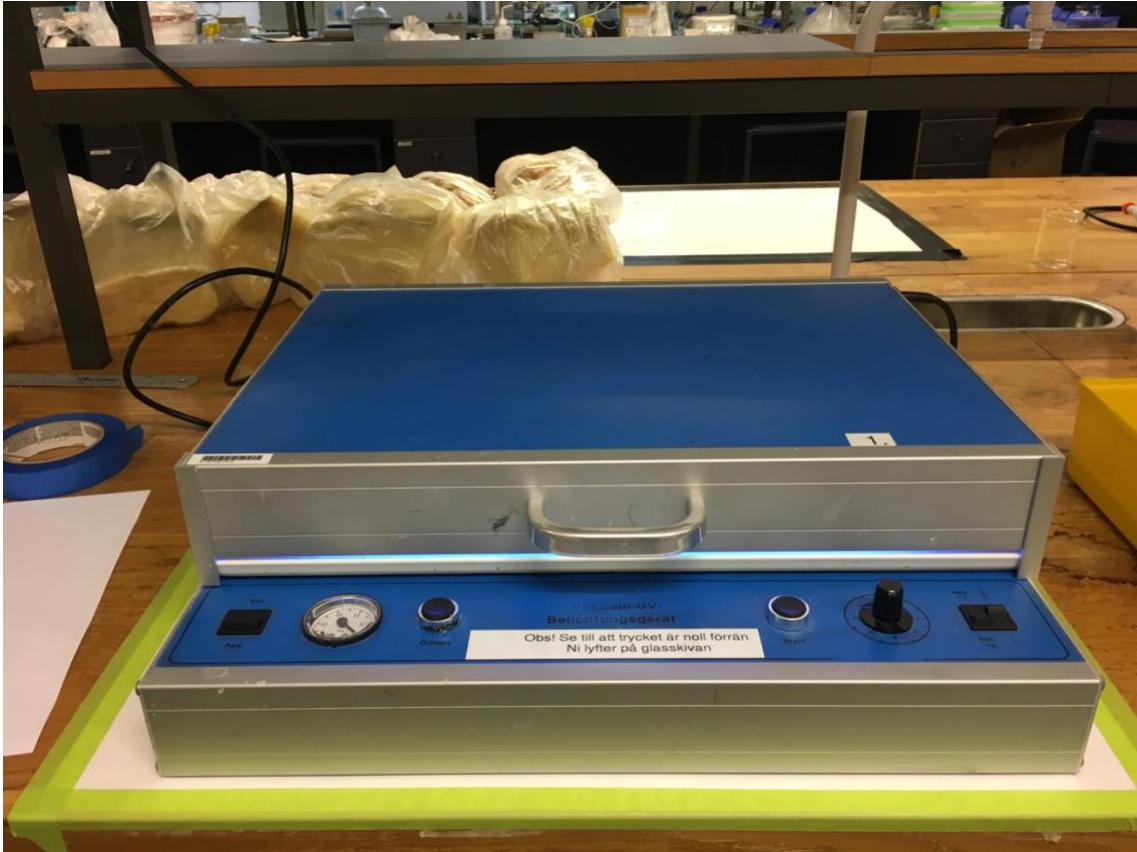
Figure 18. Photolithography Instrument transferring the pattern using UV rays
