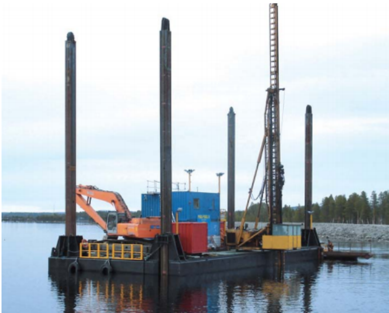
Picture 18: Semi-floating drill barge Pora-Pekka 4 (TerramareBoskalis, 2017).
