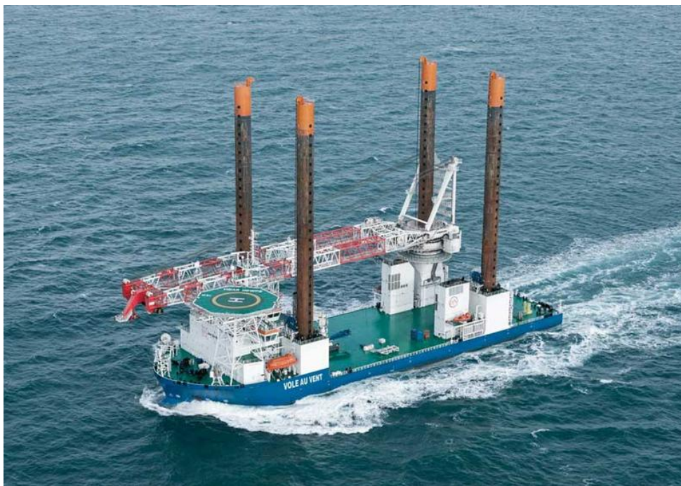
Picture 25: Turbine installation vessel Vole Au Vent (JanDeNul, 2018).
