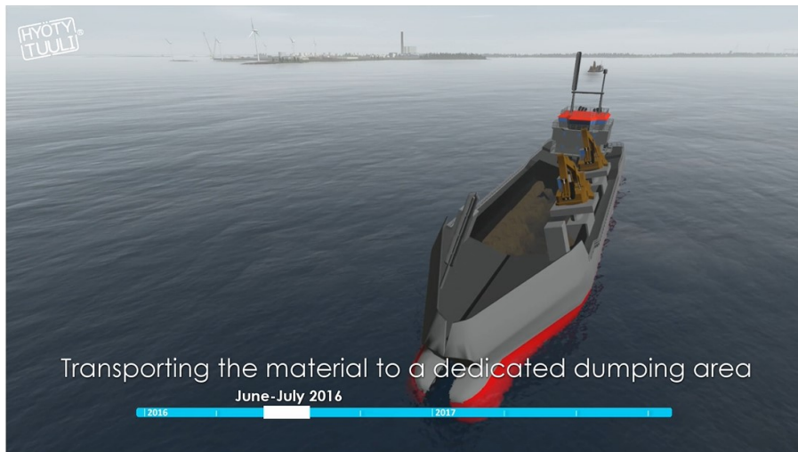
Picture 22: Split hopper barge Tiger at the dumping area (Hyötytuuli, 2017).
