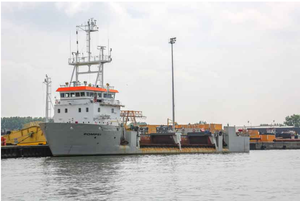
Picture 23: Stone installation vessel Pompei (JanDeNul, 2018).
