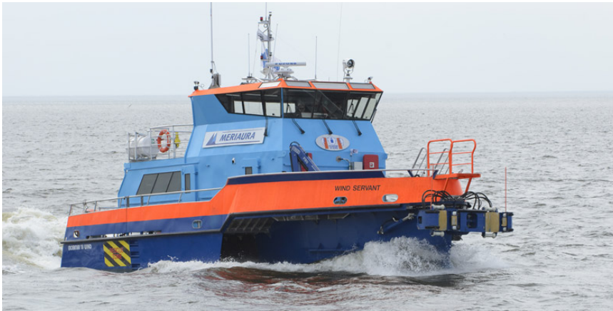
Picture 26: Wind Servant, a purpose-made vessel capable of attaching itself to the wind turbines (Auramare, 2017).
