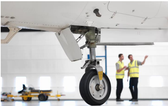
Figure 1. The real example of crank-rocker is landing gear of airplane wheel
