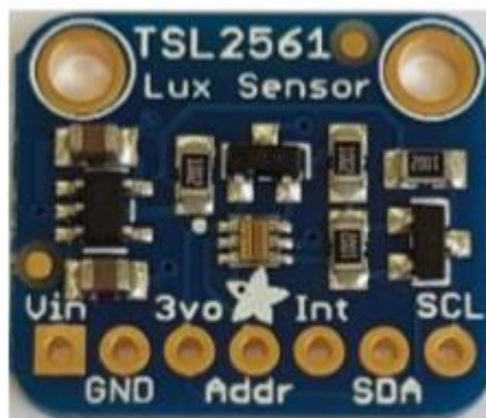
Figure 7. TSL2561 Lux Sensor.
