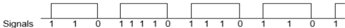
Figure 14. The Function of on/off Signals Detected by Measuring the Light and Switching Light Sensor.
