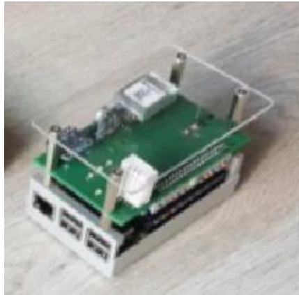
Figure 6. Room Climate Monitor.
