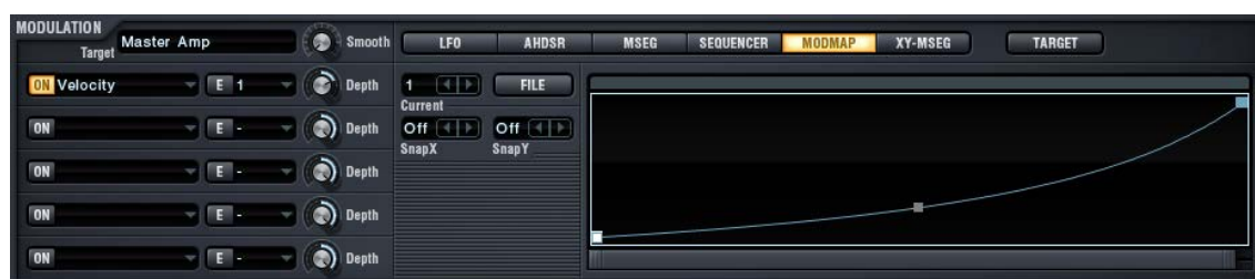
FIGURE 19. Velocity value mapped to master volume through a transfer curve in Camel Audio's Alchemy (Vuolevi 2018)
