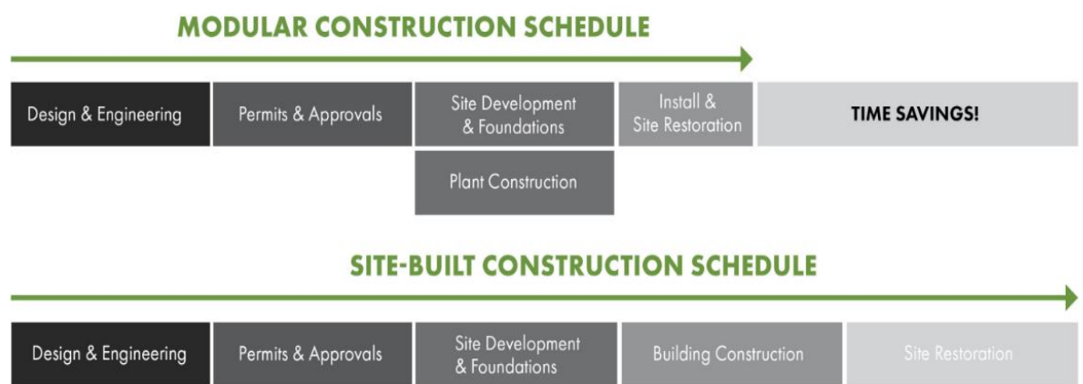
FIGURE 4. Timeline comparison of Modular and Site-built construction. (modular.org 2018)
