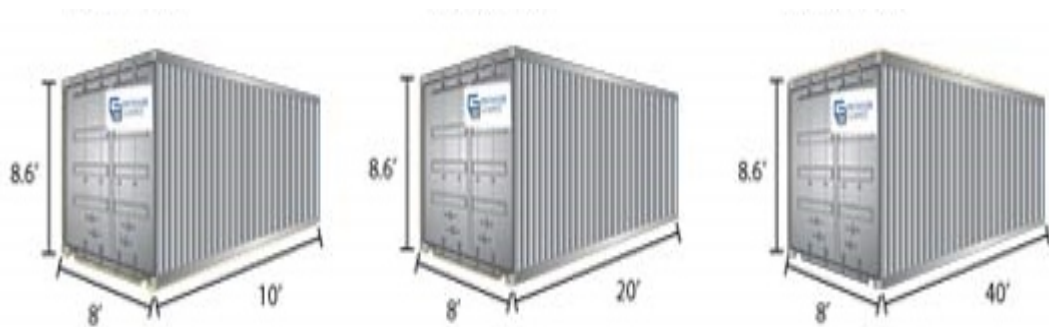
FIGURE 2. Common global Container sizes: the 10ft (3m in length), 20ft (6m in length), 40ft (12m in length) with same height of 8.6ft (2.6m) for all. (Tivacom.com 2018, modified)
