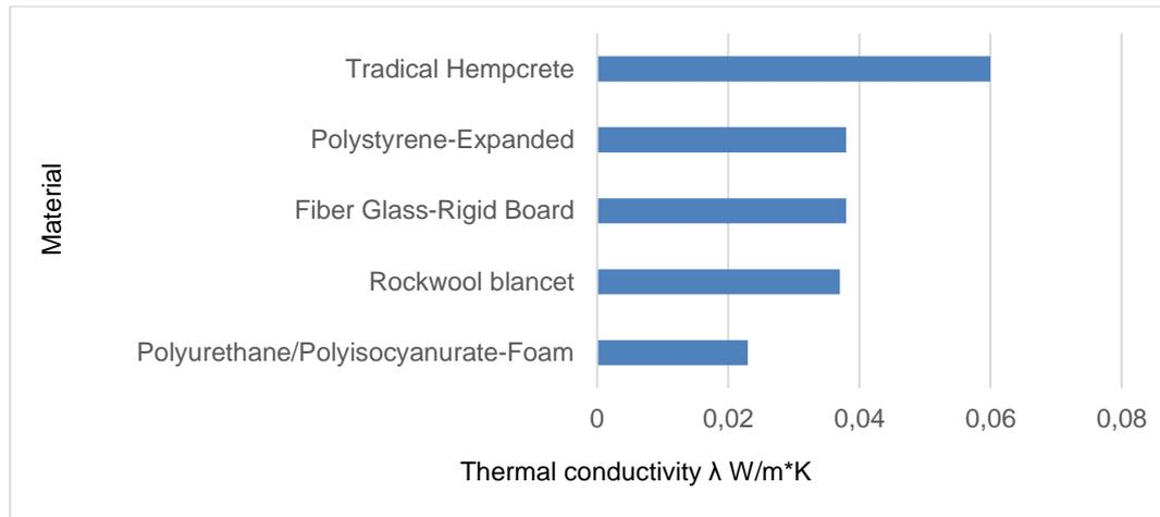
Figure 4. Thermal conductivity values for some common building materials [13,362-363; 8].
