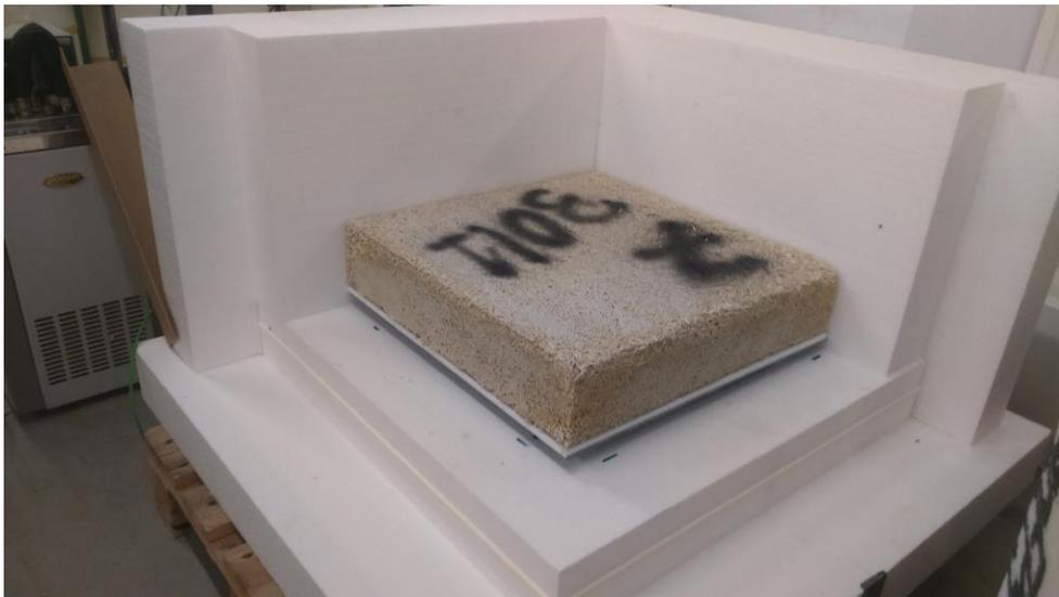
Figure 5. A sample of hemp-lime-gypsum block in the opened testing box, before testing.
