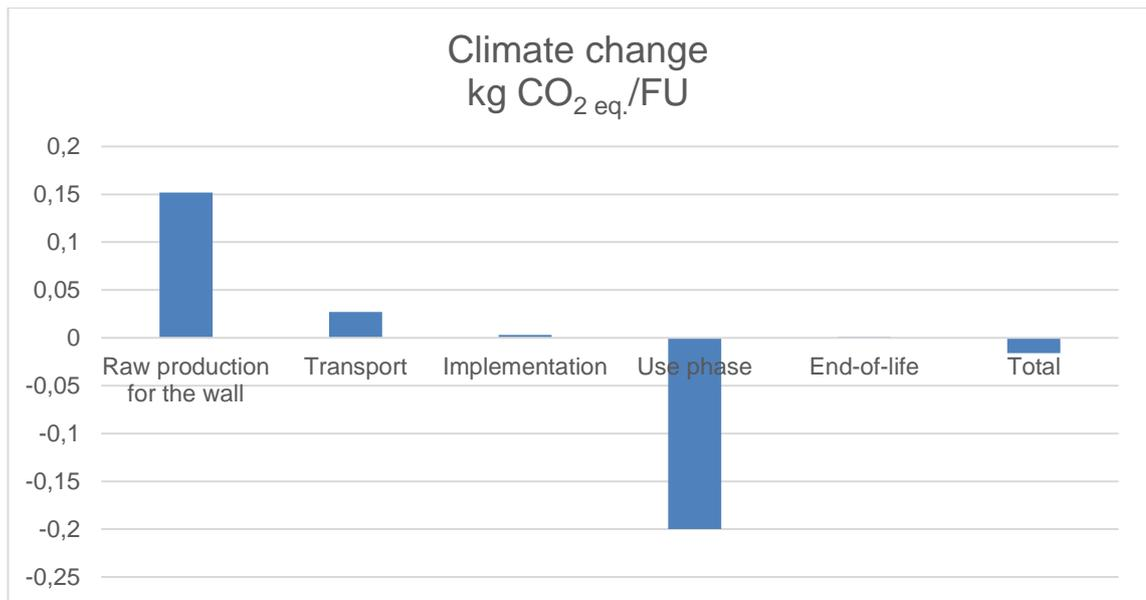
Figure 3. The distribution of CO<sub>2</sub> emissions in hemp-lime wall [6,228].
