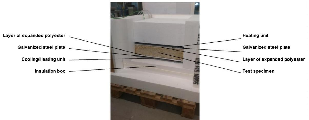
Figure 6. The testing apparatus opened from one side with explained layers.
