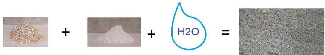
Figure 2. The elements of hempcrete and the result (sprayed hemp-lime wall)
