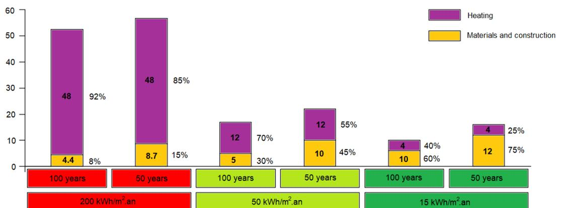
Figure 1. The deviation between the energy used in the construction phase and the energy embodied in construction materials, and the energy used in heating a conventional house. [4,31]
