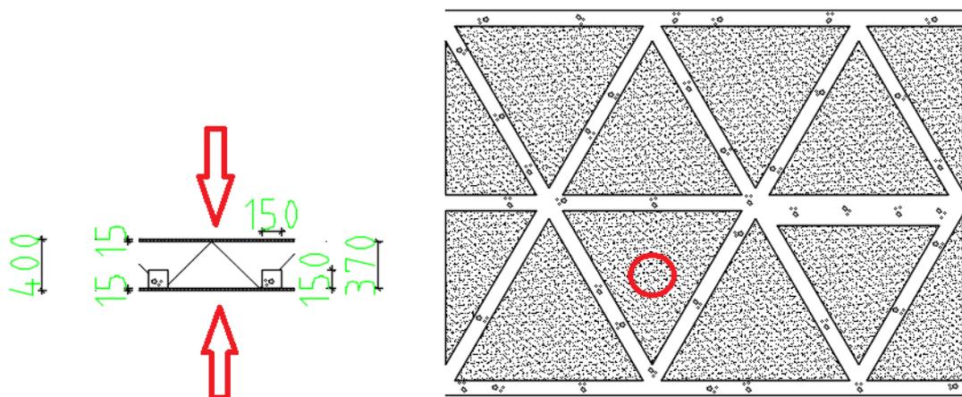
Figure 7 A sketch of the measured wall, with the sensor positions. The wall is hempcrete with lightweight concrete framework and lime render.
