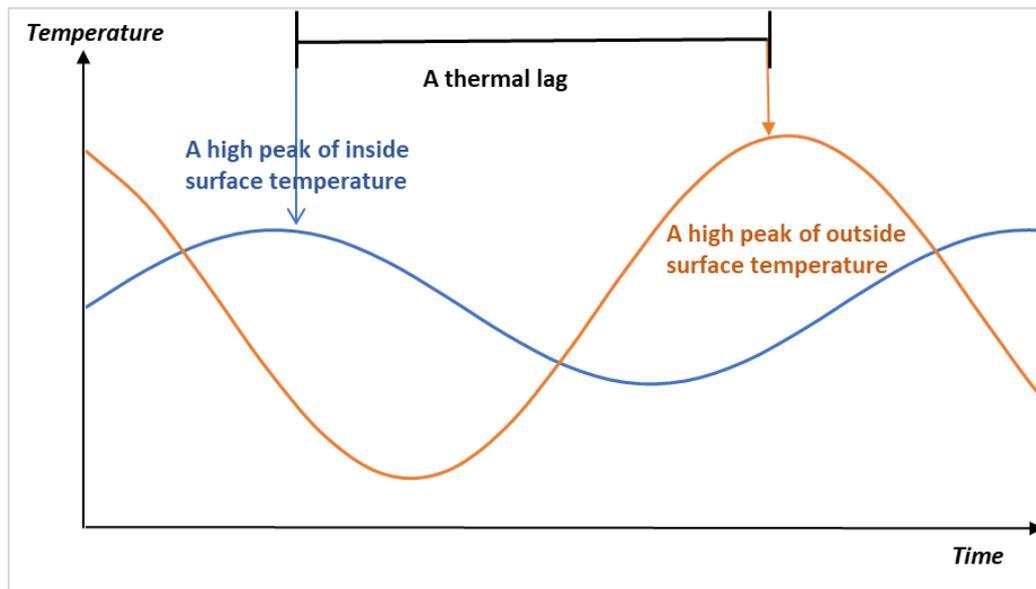
Figure 8 A simplified case of determination of thermal lag
