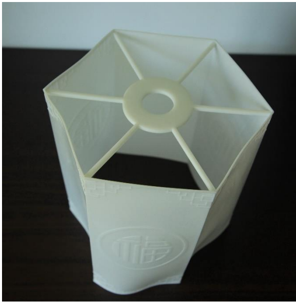
Figure 33. The deformation of the lamp shade printed with photosensitive resin, under the high temperature of summer[48]
