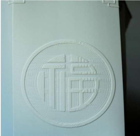
Figure 14. The rough finished surface of E-W Lantern printed by LinkeFab F500A [26]
