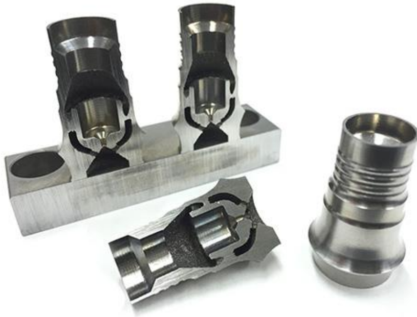
Figure 15. Engine nozzle in as build state with complicated geometry produced by Matsuura hybrid machine
