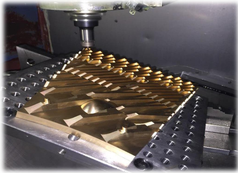
Figure 1. Manufacturing of refiner segments with traditional methods
