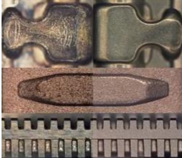
Figure 11. Metal part before and after shot peening (Nonabrasive Cleaning N.d.)
