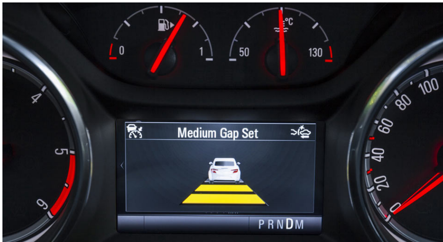
Figure 7. AAC automatically adjust speed to keep a pre-set distance to traffic ahead (Gnaticov 2016)
