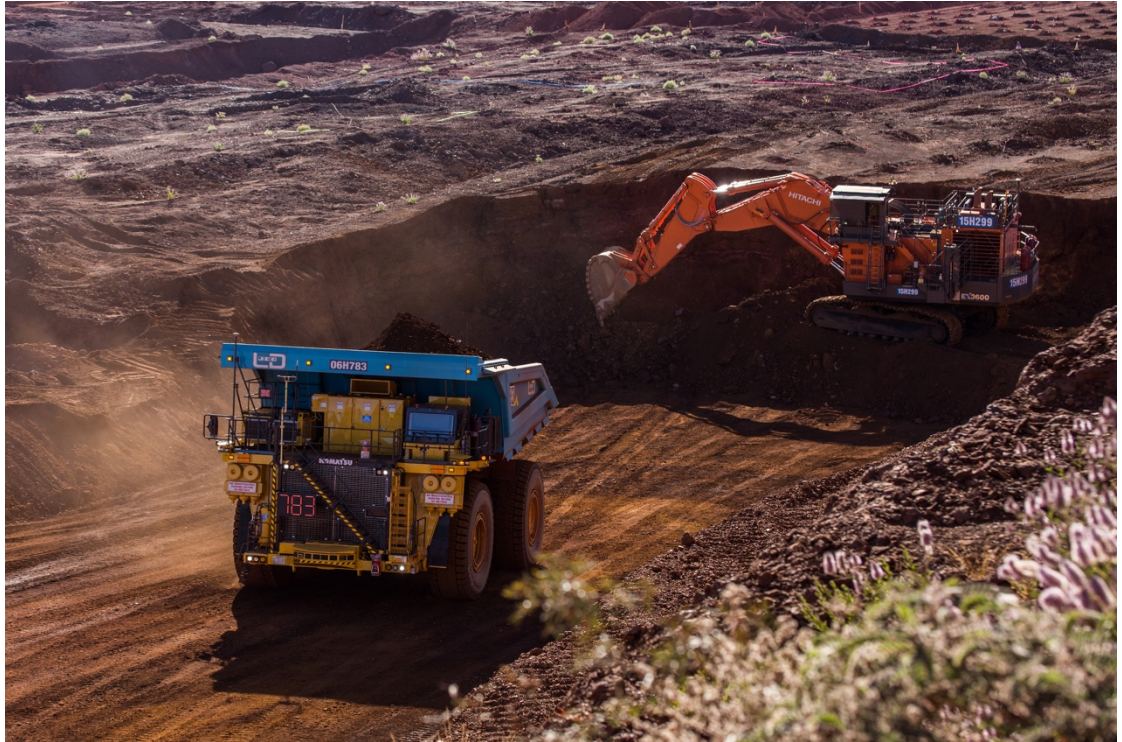
Figure 5. Autonomous haul trucks in mining industry (Rio Tinto Photo Library 2017)
