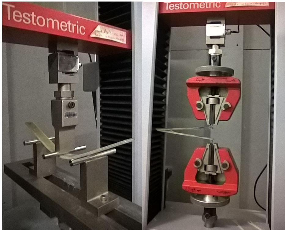
Figure 19: 3 point bending test (left) and Peel test (right)
