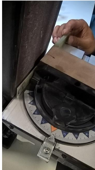
Figure 16: Sanding process using jig
