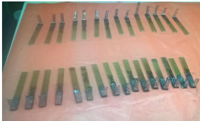
Figure 20: Preparation of peel test samples
