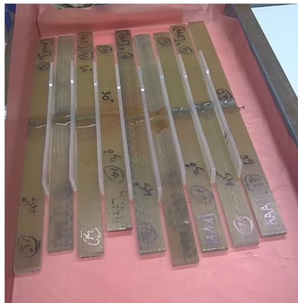
Figure 18: Bonding of scarf joint UD laminates
