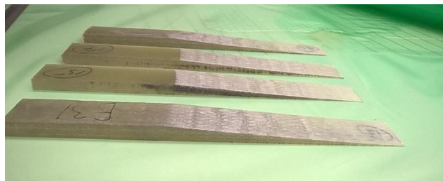
Figure 17: Sanded 86° scarf angle UD laminate
