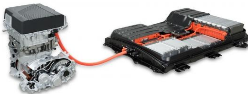
Nissan Leaf 2018 - traction drive and battery pack
