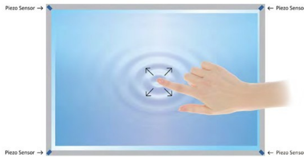
Kuva 17. Dispersive signal technology (TouchSystems Corporation 2016 C).
