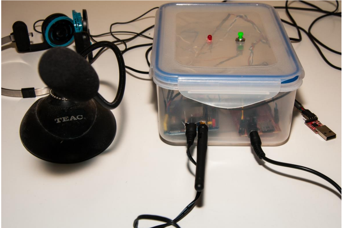
Figure 13 - The final proof of concept setup. On the left side the microphone and headphones for verifying the GSM call. The user panel can be seen on top, with the button to answer and initiate a call, and the LED as an indicator for user feedback.
