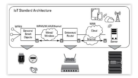
Figure 4. IoT system architecture and functional overview (Miller 2016, 6)
