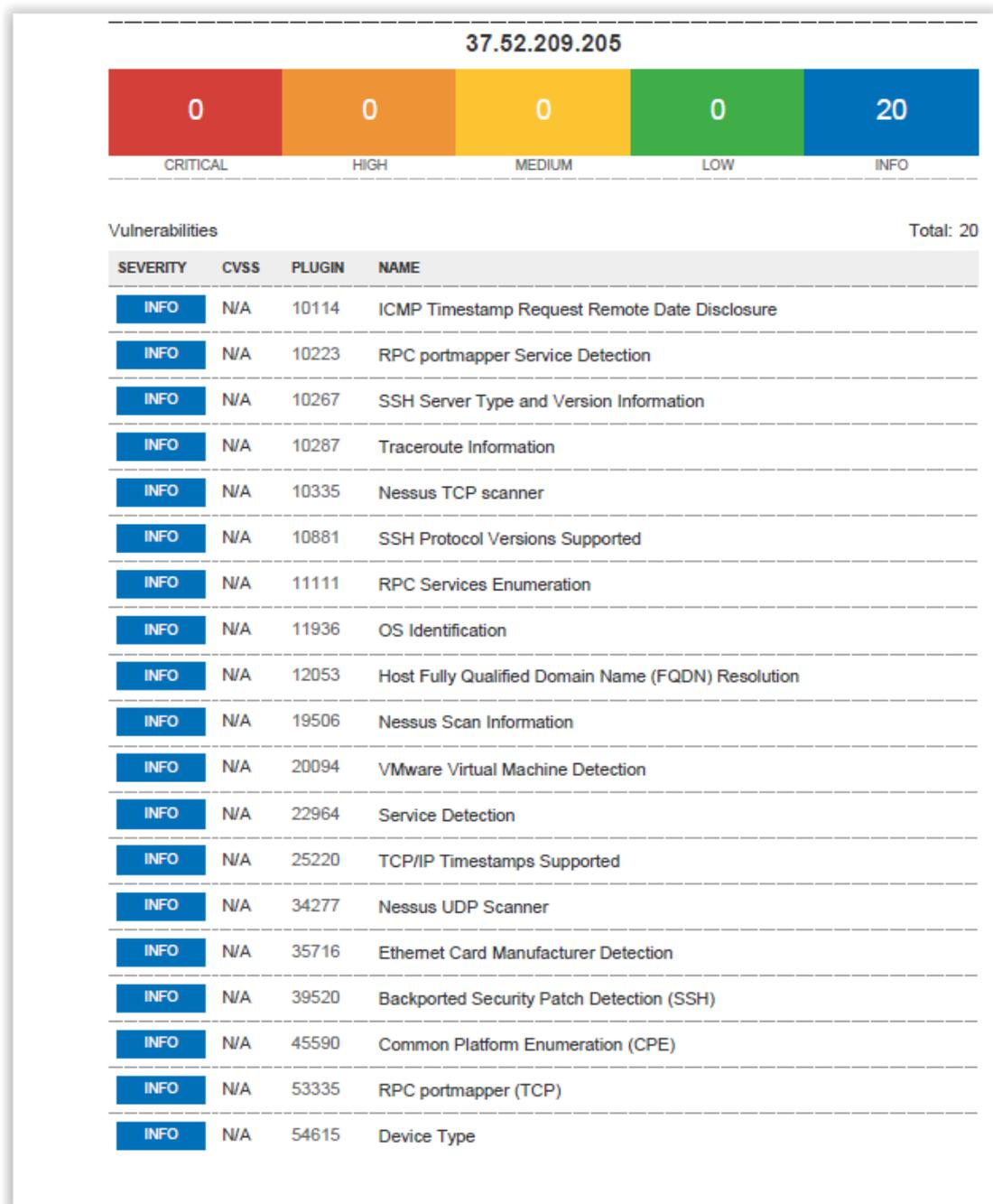
Figure 22. Sensor AMQP Nessus Advanced scan result
