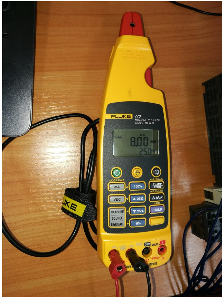
Figure 14. Fluke 773 Process Meter with milliamperere transmitting functionality (Samuli Multaniemi, 2018)
