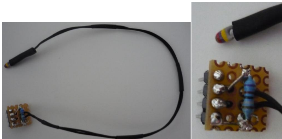
Figure 17. Improved Circuit Board for the NTC Thermistor [own figure]
