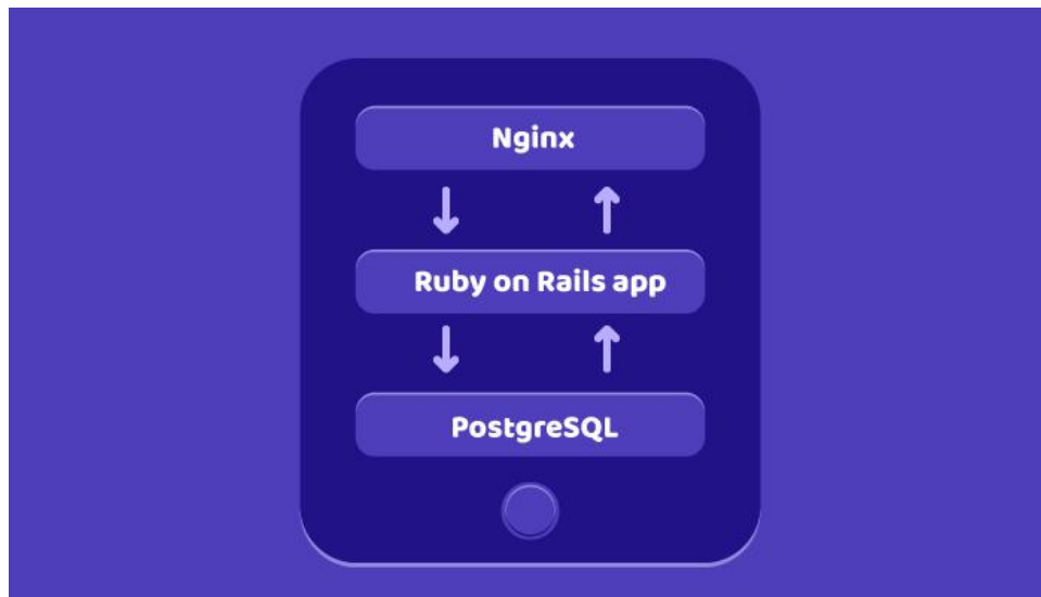
Figure 3 Single tier server architecture (Source : https://rubygarage.org/blog/ruby-on-rails-is-scalable )
