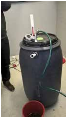
Picture 15. Fully loaded and sealed reactor, with temperature analyzer (picture: Kari Laasasenaho).
