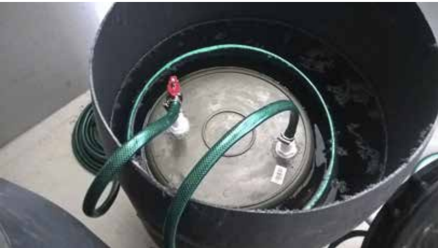
Picture 13. If the gas collector is going to skewed position, extra frame can be installed (picture: Kari Laasasenaho).
