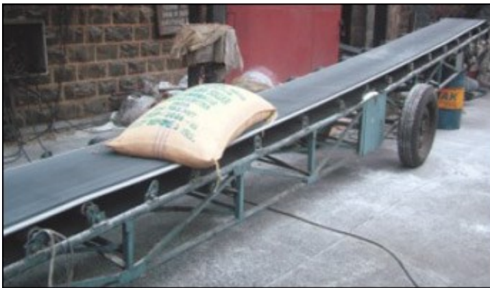
Figure 9. Belt conveyor with a single bag conveyed (Rollcon, n.d.)
