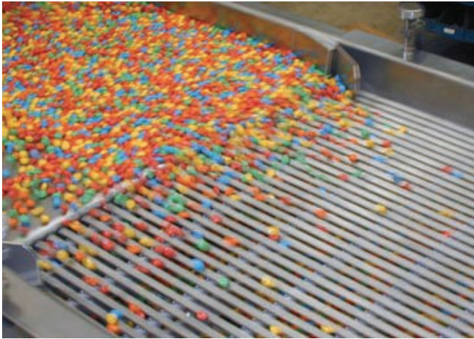
Figure 8. Screening with vibratory conveyor (Meyer n.d.).
