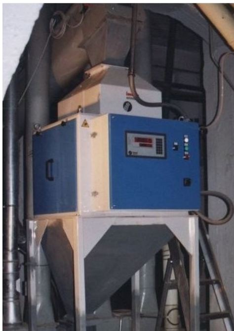
Figure 27. Imeco Weighing Hopper connected to tank directly (Imeco n.d.).
