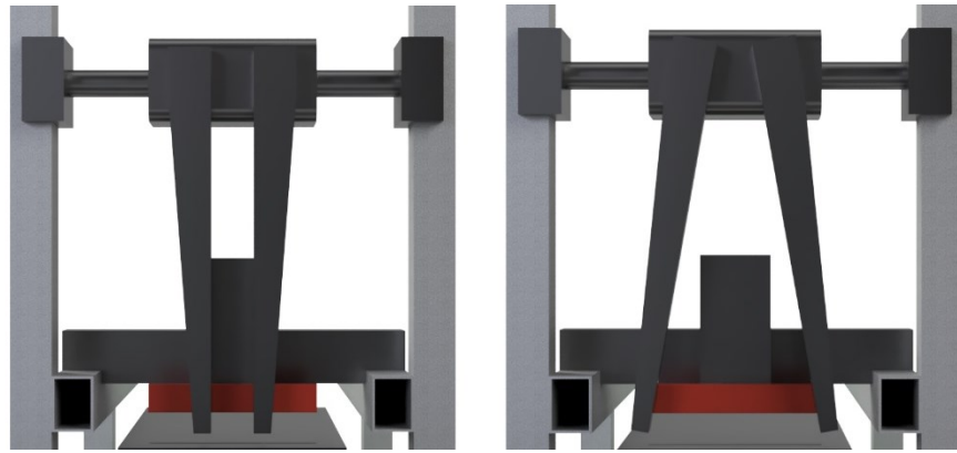
Figure 45. Fork mechanism concept (Mehta Heino Industries Oy 2018).
