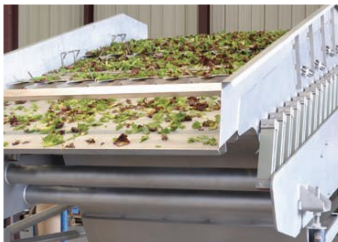
Figure 7. Horizontal transfer with vibratory conveyor (Meyer n.d.).
