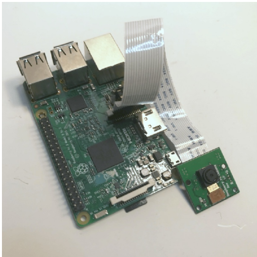
Figure 18. Mounting the camera module to the Raspberry Pi
