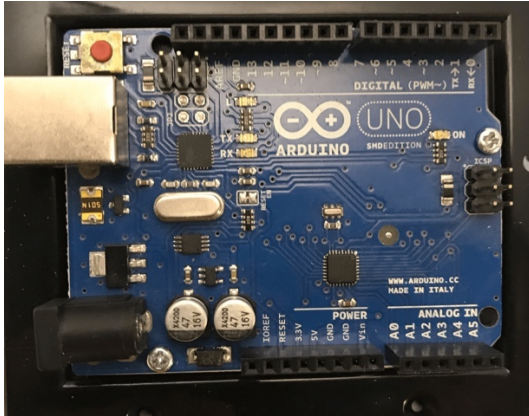
Figure 8. Arduino Uno microcontroller board
