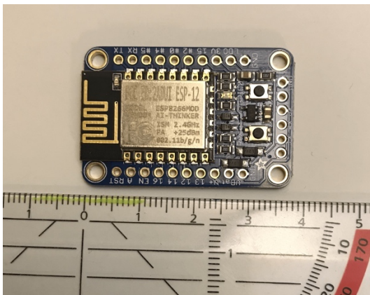
Figure 9. Adafruit Huzzah Breakout ESP8266
