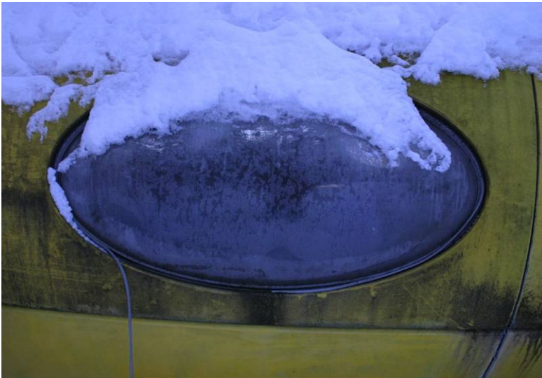
Figure 113. Window seal is loose.
