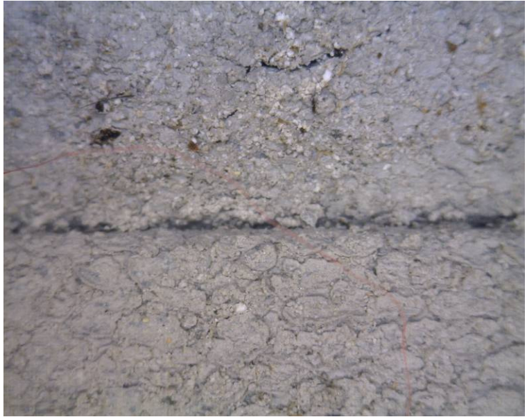
Figure 111. Ice on the window seal. Figure 112. Window seal surface has altered from smooth to uneven. (60-fold magnification)
