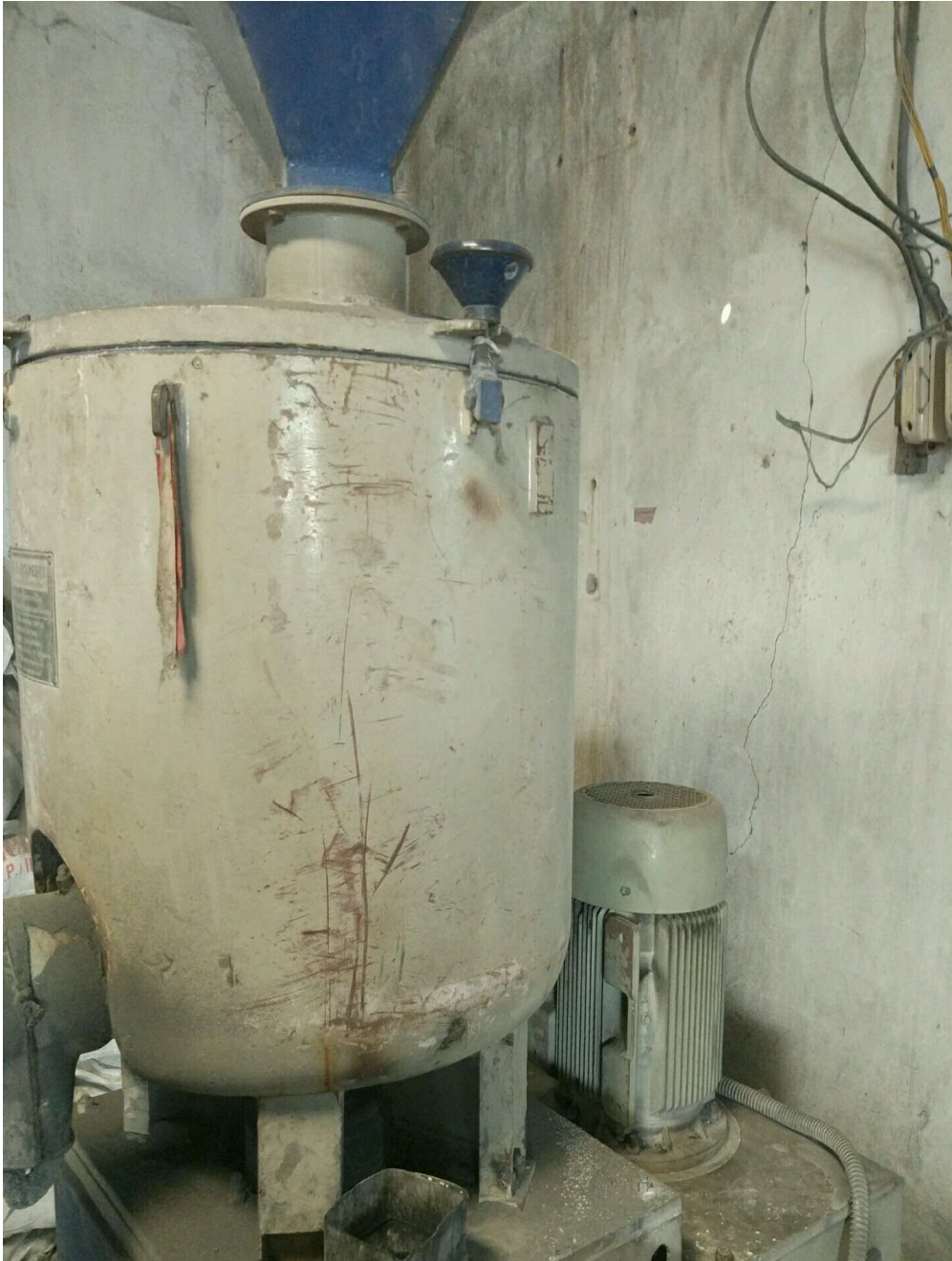
Figure 9. Drier and mixture at Seti Plastics (Nishan Devkota, 2017)
