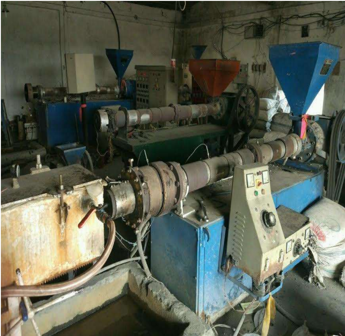
Figure 8. Pipe extruder machine at Seti Plastics (Nishan Devkota, 2017)
