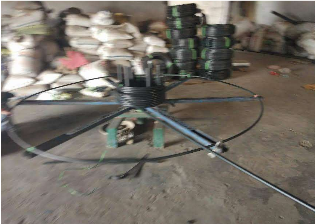
Figure 20. Winding machine and rolling a HDPE pipe at Seti Plastics (Nishan Devkota, 2017)
