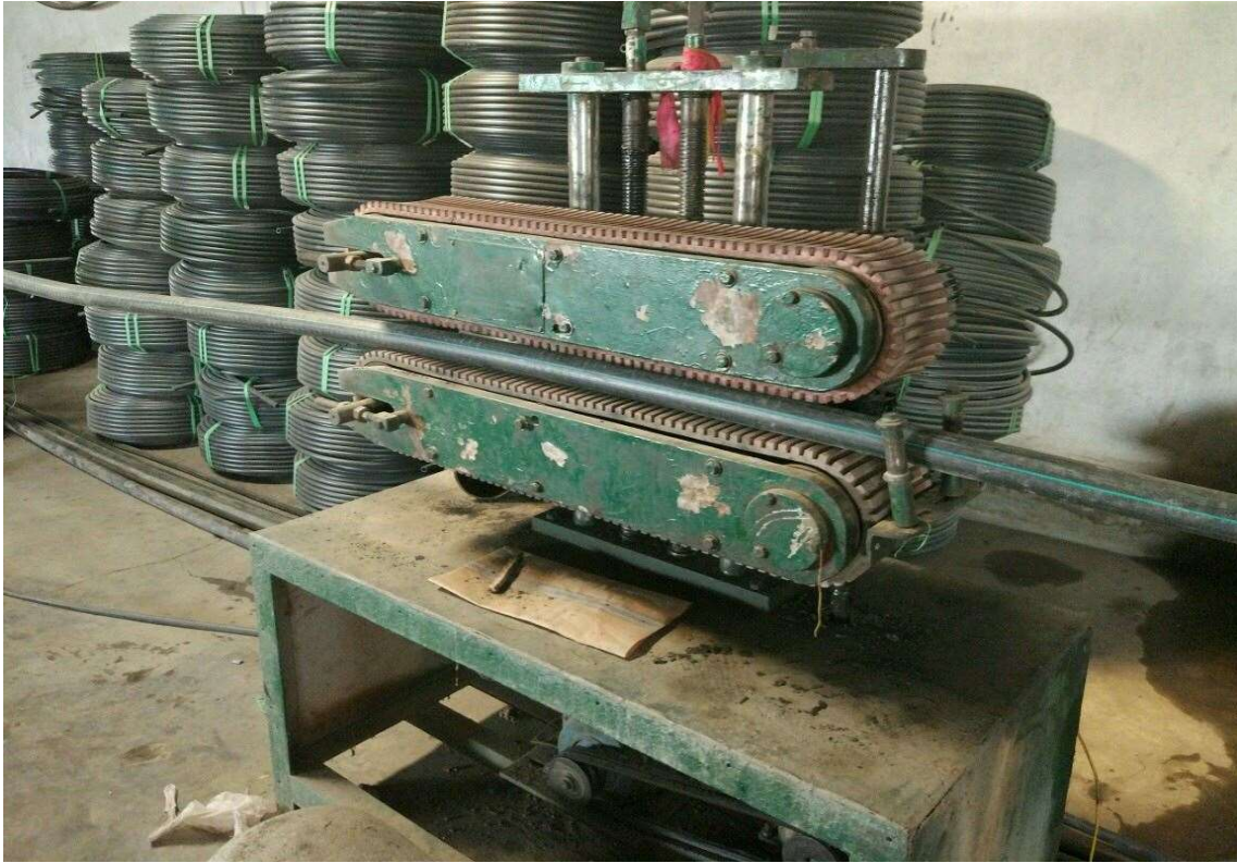
Figure 17. After cooled in bathtub at Seti Plastics (Nishan Devkota, 2017)
