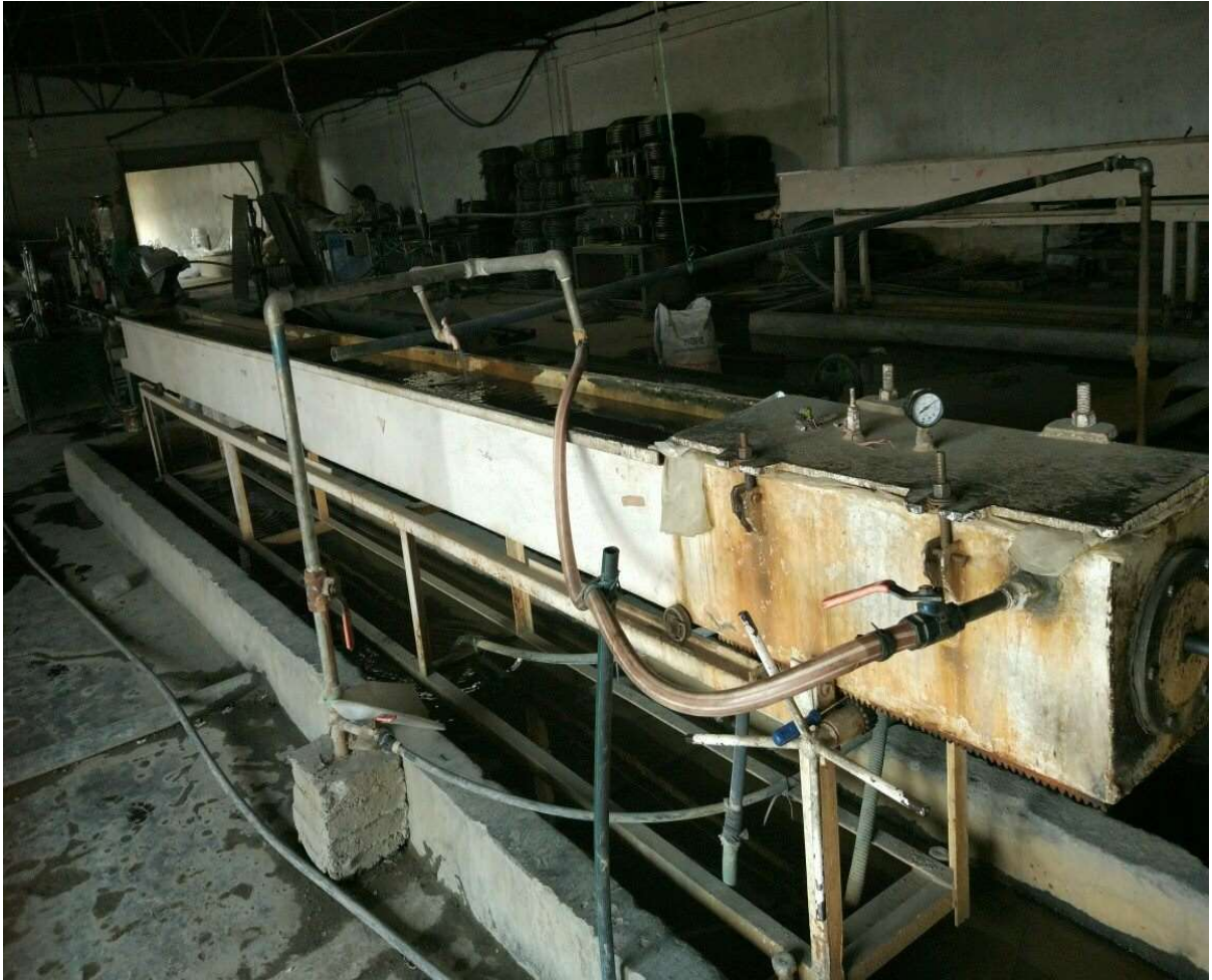
Figure 16. Six-meter water bathtub at Seti Plastics (Nishan Devkota, 2017)
