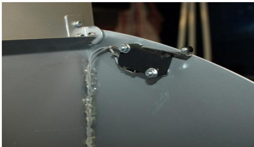
Figure 8: detection switch inside a mailbox
