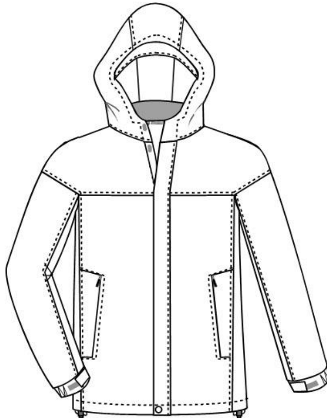
Figure 11: Flat drawing of a jacket showing the stitch type, shape and trims of the apparel (Clothier Design Source 2006)
