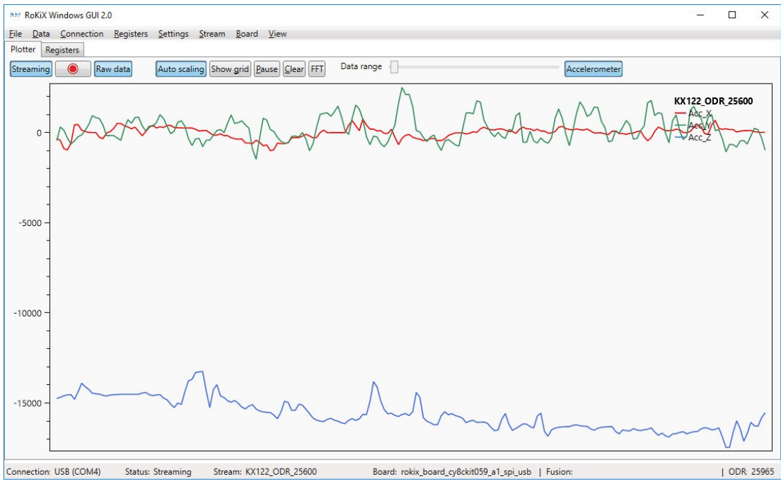
FIGURE 3. 3-axis acceleration data at 25.6 kHz output data rate (ODR) in RoKiX Windows GUI's plotter-view.
