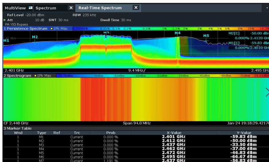
Figure 54. Second real time spectrum analyzer measurement results for microwave oven interference signals. Four meters distance between measurement antenna and microwave oven.
