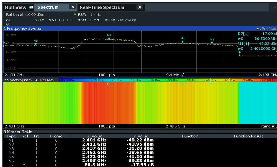
Figure 57. Second swept tuned spectrum analyzer measurement results for Bluetooth loudspeaker interference signals. Four meters distance between measurement antenna and Bluetooth loudspeaker.
