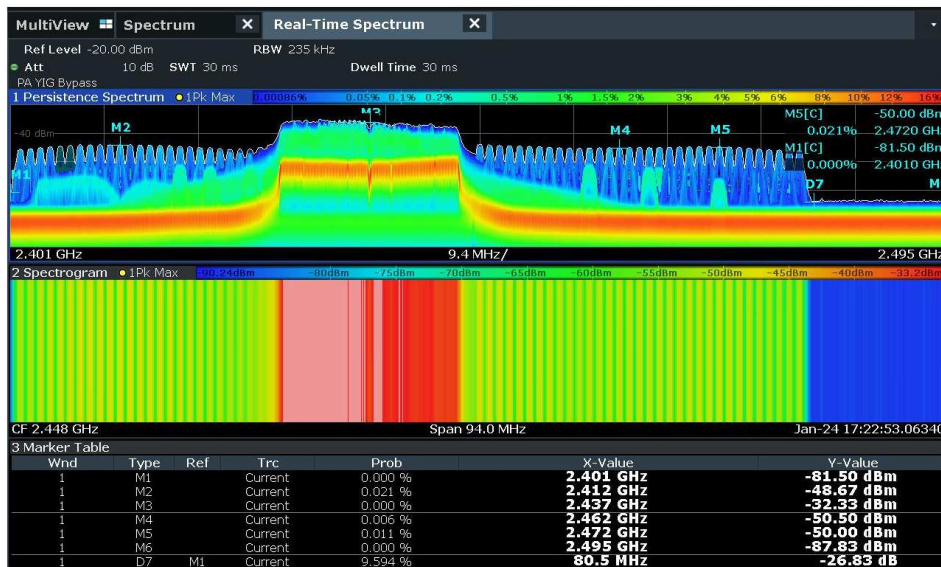
Figure 58. Second real time spectrum analyzer measurement results for Bluetooth loudspeaker interference signals. Four meters distance between measurement antenna and Bluetooth loudspeaker.
