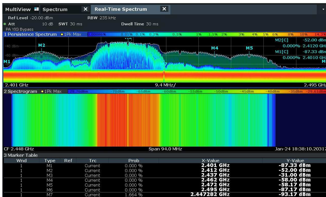
Figure 39. Real time spectrum analyzer reference measurement results for experimental WLAN network. Two meters distance between measurement antenna and WLAN access point.
