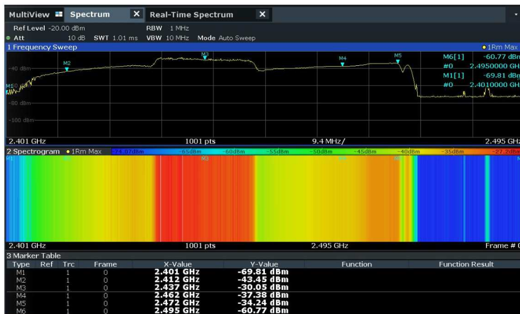
Figure 41. First swept tuned spectrum analyzer measurement results for microwave oven interference signals. Three meters distance between measurement antenna and microwave oven.
