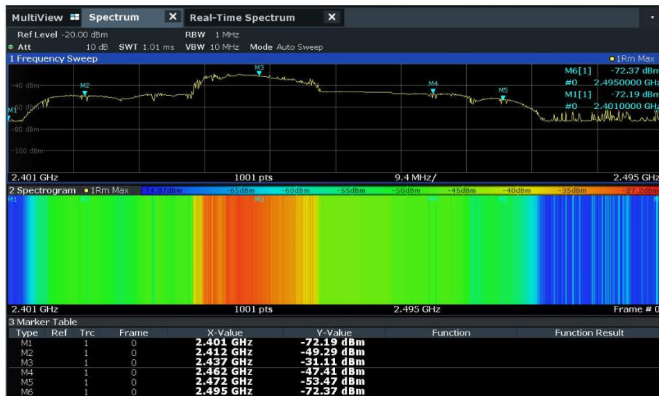
Figure 55. Third swept tuned spectrum analyzer measurement results for microwave oven interference signals. Five meters distance between measurement antenna and microwave oven.
