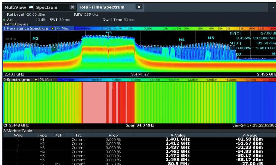
Figure 60. Third real time spectrum analyzer measurement results for Bluetooth loudspeaker interference signals. Five meters distance between measurement antenna and Bluetooth loudspeaker.
