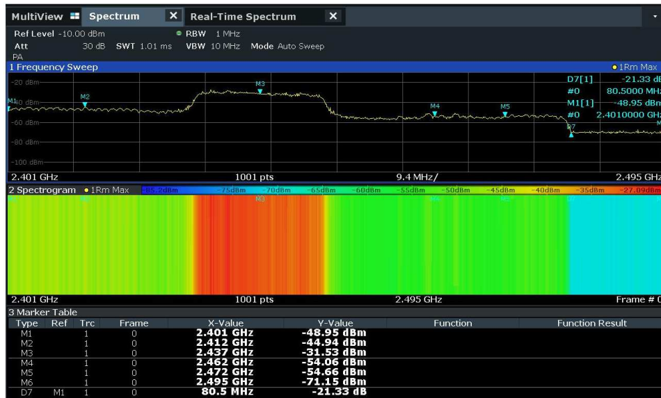
Figure 59. Third swept tuned spectrum analyzer measurement results for Bluetooth loudspeaker interference signals. Five meters distance between measurement antenna and Bluetooth loudspeaker.
