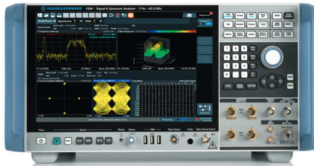
Figure 33. Front view of FSW 26 spectrum analyzer. [27; p.2]
