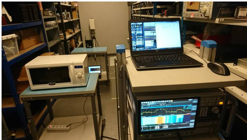
Figure 40. Test setup for microwave oven interference measurements.
