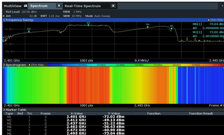
Figure 53. Second swept tuned spectrum analyzer measurement results for microwave oven interference signals. Four meters distance between measurement antenna and microwave oven.
