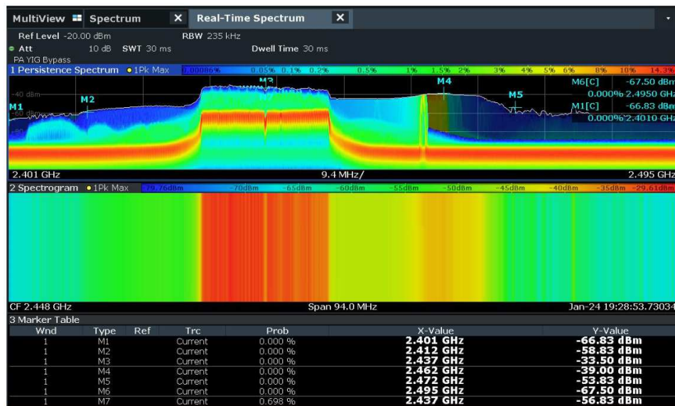
Figure 56. Third real time spectrum analyzer measurement results for microwave oven interference signals. Five meters distance between measurement antenna and microwave oven.
