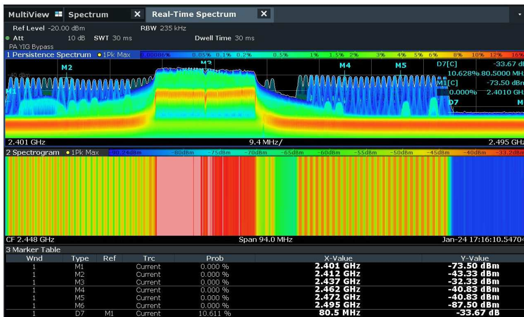
Figure 45. First real time spectrum analyzer measurement results for Bluetooth loudspeaker interference signals. Three meters distance between measurement antenna and Bluetooth loudspeaker.
