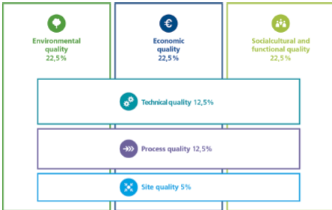
Fig. 6 The Basic Structure of DGNB System showing the 6 categories and their weights in %
