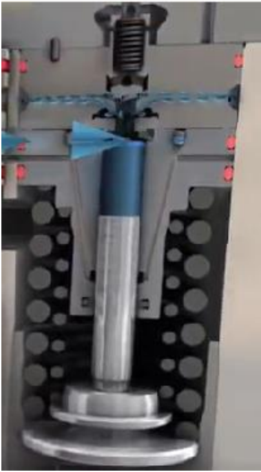
Figure 7. Suction stroke of L'Orange multi plunger pump. /12/
