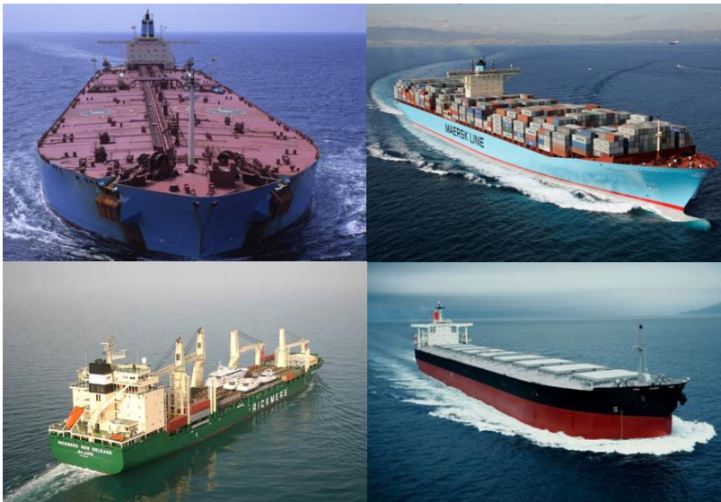
Figure 4. Figure shows a Crude Oil Tanker (top left), Container Vessel (top right), General Cargo Vessel (bottom left), and a Bulk Carrier (bottom right). (Wärtsilä 2018f)
