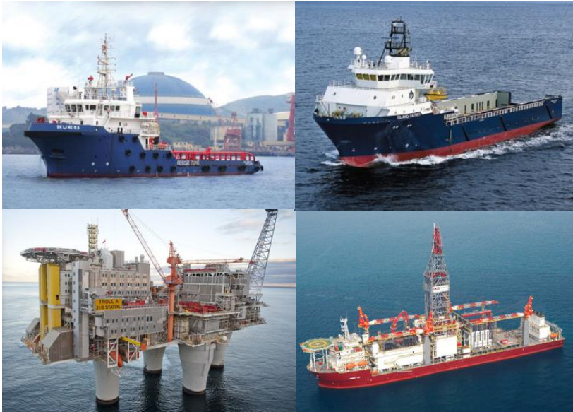
Figure 5. Figure shows an Anchor Handling Towing Supply Tug AHTS (top left), Offshore Supply Vessel (top right), Fixed Production Platform (bottom left), and a Drillship (bottom right). (Wärtsilä 2018f)
