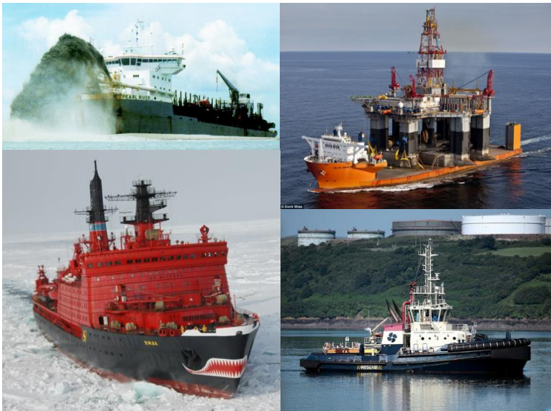
Figure 7. Figure shows a Dredger (top left), Semi-submersible heavy lift vessel (top right), Icebreaker (bottom left), and an Escort tug (bottom right). (Wärtsilä 2018f)
