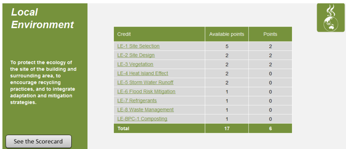
Figure 61. LOTUS assessment system results of the Local Environment category for the Alpes building
