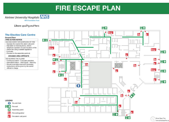
Figure 16. Emergency exit plan of a hospital (Firesafe, 2011)
