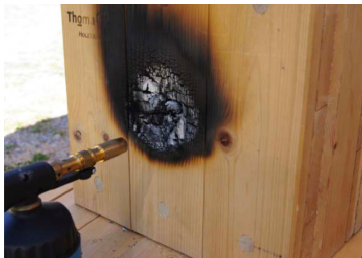
Figure 21. Damage after 60 min, on a solid wood OWE (Petersen, Rödel, (2014). p.16)
