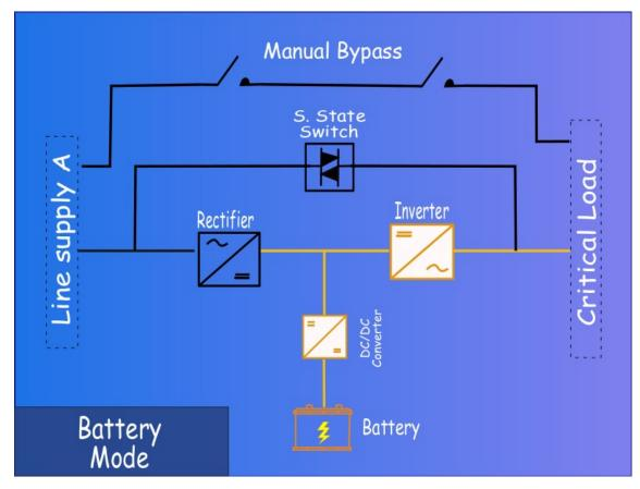
Figure 16. Battery mode during power failure or outage.
