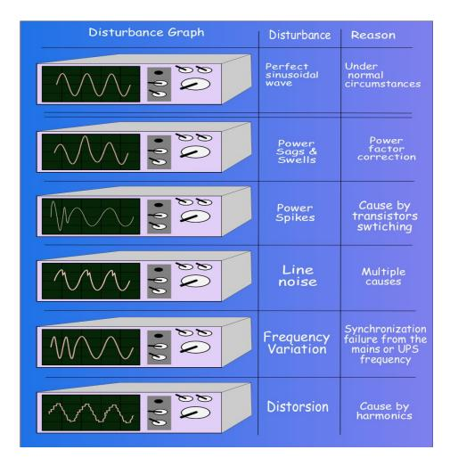
Figure 8. Typical disturbances generated by UPS system.[10]
