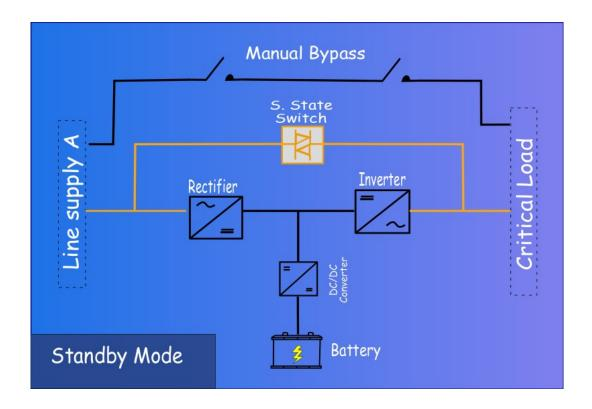
Figure 14. Power flow of Passive Standby Mode or VFD.
