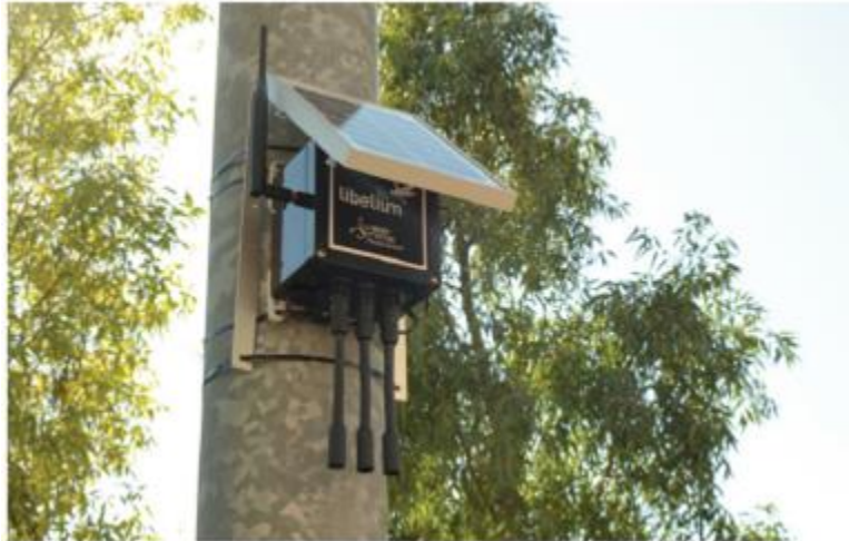
Figure 14. Wasmote Plug and Sense! being powered by an external solar panel [32]
